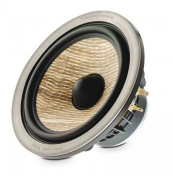
It has an inverted dome made of magnesium-aluminium alloy, supposedly to increase damping and rigidity. The suspension uses Poron, a material with shape memory. Focal says this improves control.
